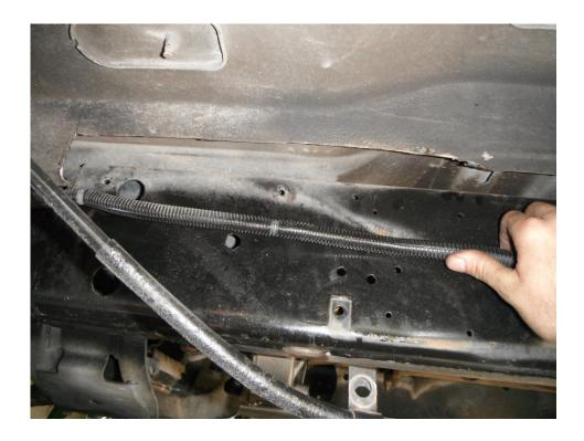
Locate the stock transfer case skid plate cross bracket, that runs from driver side to passenger side across the frame. Remove it from each side of the frame and discard. You will not be reusing this.
