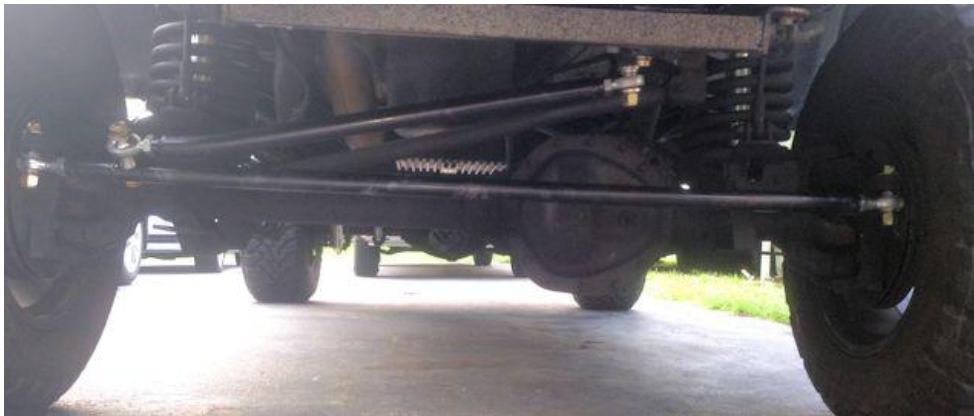
DOR Heavy Duty T-Style Steering Linkage, the only aftermarket bolt-in steering kit in the world!
