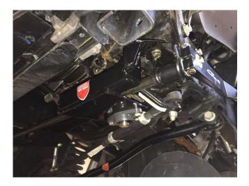
Once the brace is in position, you can begin to align it with the bolt holes. The easiest way to do this is to put the steering box bolt through the side tab on the brace and thread it in a couple of turns, and then you can either push up on the sway bar bushing mount, or use a floor jack to raise the sway bar into position. Once you are able to get the new bolts started by hand, you can tighten them, but do not torque them yet. The new bolts will take a 17mm socket.
