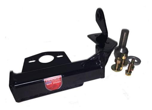
Thank you for purchasing our patented Dodge Off Road Steering Brace, the strongest and bestdesigned steering brace on the market for Dodge Ram trucks! This brace is used to support your steering box from the push and pull design of Dodge steering, while eliminating the transfer of frame flex to the sector shaft, which is a problem that all frame-to-frame braces cause.
