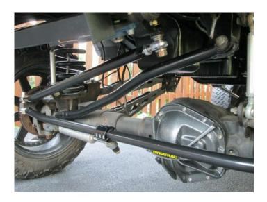
Please recheck all hardware after 100 miles, as the bolts can stretch. Recheck as needed afterwards. Trucks used in harsh conditions such as gravel roads, poorly maintained roads, or in off road environments, should recheck hardware more frequently. It is up to the owner of the truck to ensure all hardware is securely tightened and remains tight as part of your truck maintenance.
