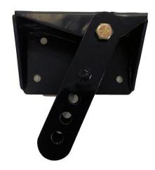
Installation of the shackle flip kit requires your stock shackle plate to be removed. If this is done properly, the plate can be reused later if you wish to return to stock. There are no permanent modifications required, as the new bracket bolts up to the existing holes in the frame.
