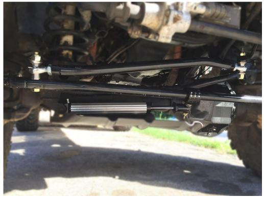
Steering installed in a 3" to 6" configuration, with the drag link below the pitman arm.
