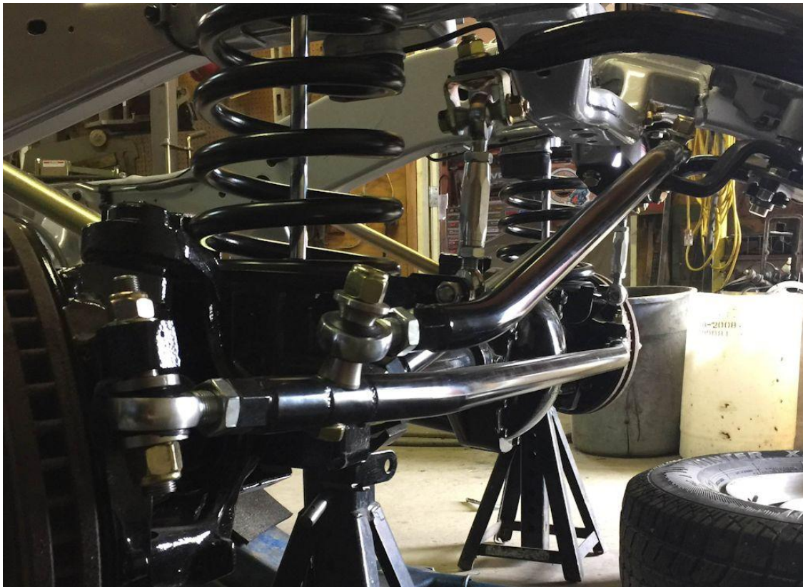
Steering installed in a stock to 3" configuration, with the drag link above the stock pitman arm.
