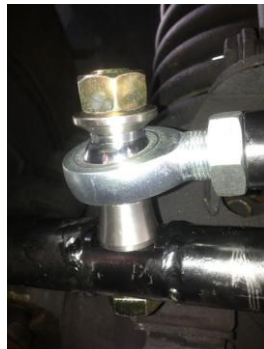
Drag link mount on the tie rod, pre-assembled
